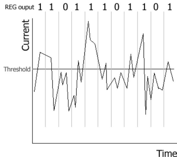
**FIGURE 3: Threshold conversion of analogue current to binary REG output**
